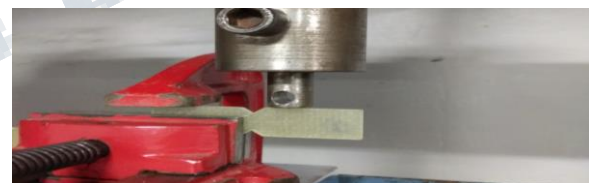
Fig. 2. Shear Testing of Composite Specimen
