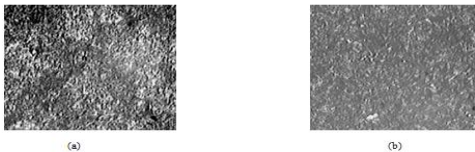
Figure 7: Optical micrographs of water quenched specimens at 250 X (a) Muffle furnace (b) Microwave oven
