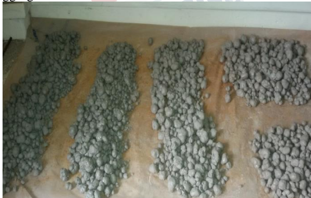
Figure 4: Air curing of the artificial aggregates
