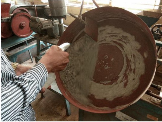
Figure 2: Spraying of Alkali Solution
