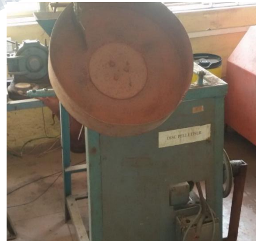
Figure 1: Laboratory disc pelletizer
