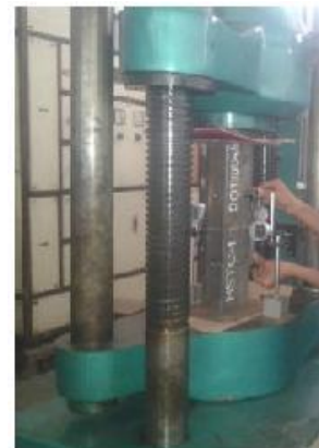
Fig 4: Test setup for testing of Hollow Steel Tubular Columns in UTM.
