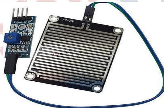
**Fig.7 Liquid sensor**
