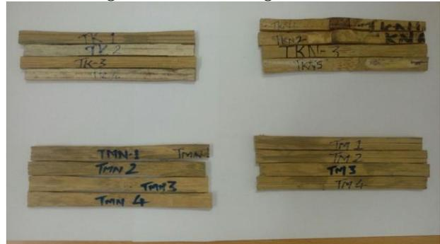
**Fig 13. Tensile test specimens**
