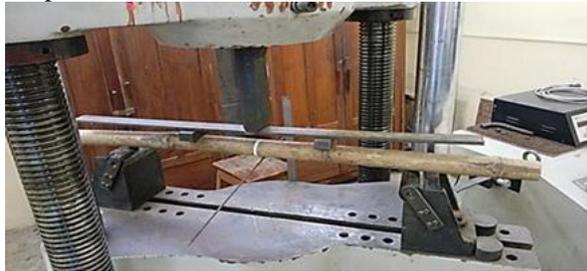
**Fig.10 Static bending test on bamboo sample**
