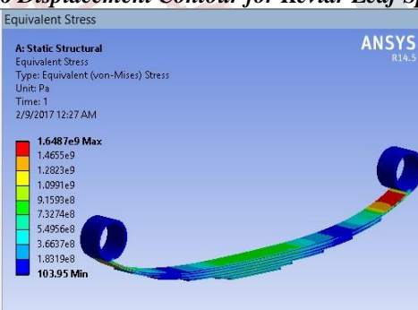
Fig.7 Von Mises Stress Distribution for Steel Leaf Spring
