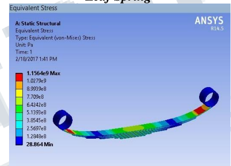
Fig.9 Von Mises Stress Distribution for Aluminium/Boron Leaf Spring
