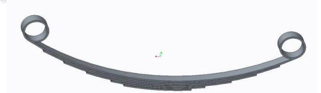
Fig. 2 Leaf Spring Designed in CREO 2.0 Environment
