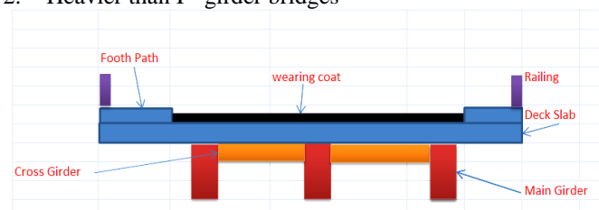
Figure 1: Cross section of T-beam bridge
