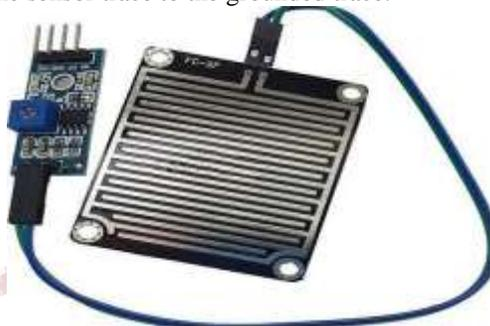
**Fig.7 Liquid sensor**
