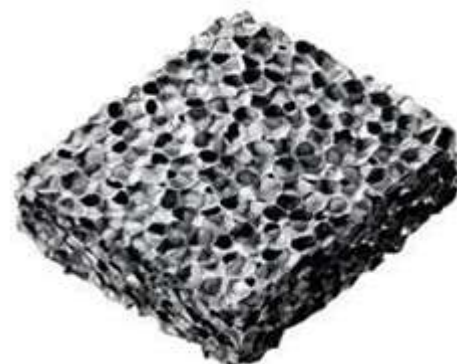
Fig : Aluminium foam- Closed cell type.
