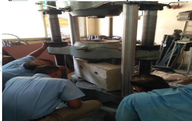
FIGURE 1: ULTIMATE LOAD TEST SETUP
