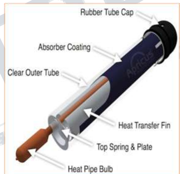
Fig.9: Cross sectional view of ETSC
