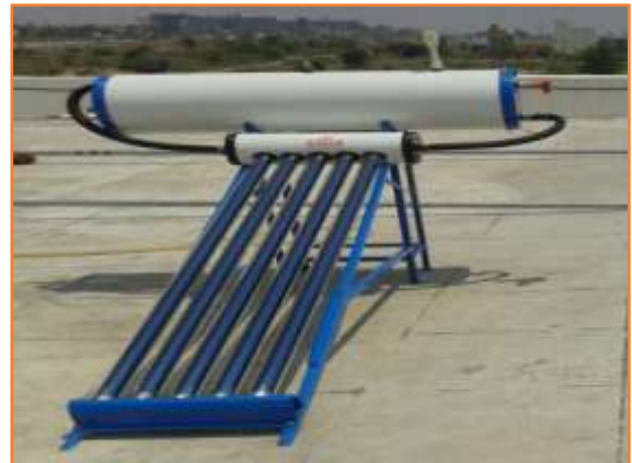
Fig.8: Setup of concentric type heat exchanger ETSC
