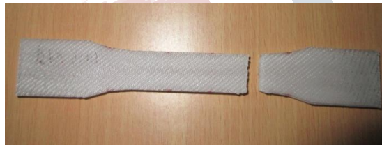
Fig 2.4: Fractured tensile specimen
