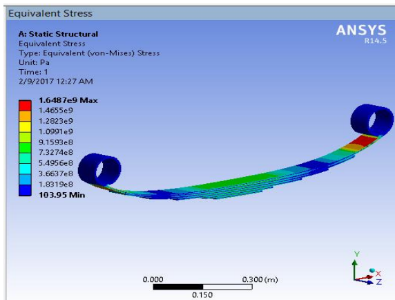
Fig 8: Von Mises Stress Distribution for Steel Leaf Spring
