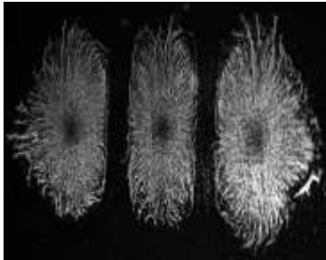
Figure.6(a) Flow distribution of painted carbon black on concave surface for H/d=2 and for Re=1769
