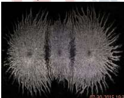
Figures 8(c): Flow distribution of painted carbon black on concave surface with H/d=4 and Re=3496
