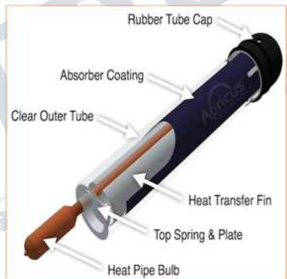
Fig.9: Cross sectional view of ETSC
