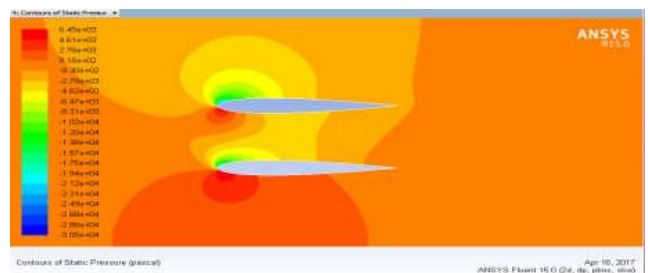
Figure 5: Contours of static pressure at 140 AOA for biplane d of 0.5 times of C
