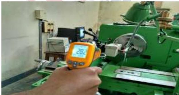
**Figure 6 MT 4 Infrared thermometer**
