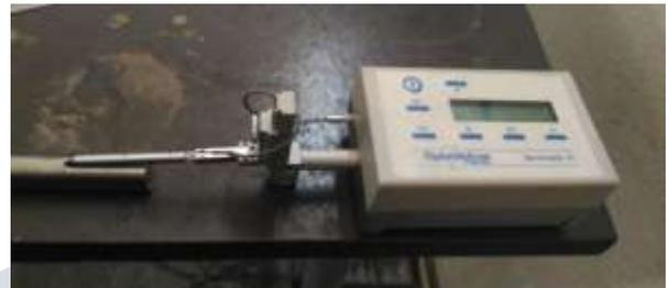
**Figure 7 Surface Roughness Tester**
