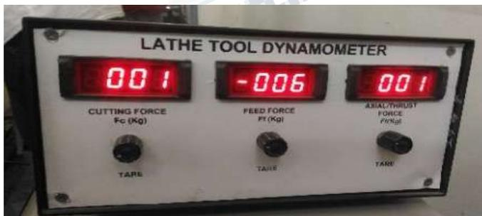
Figure 4 Lathe Tool Dynamometer
