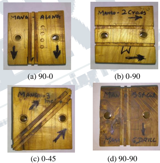
Fig 4:- Machining trials showing different interactions of tool and wood grain (for mango wood)
