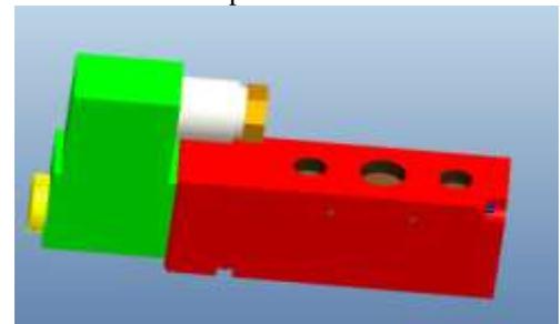
This valve was selected for speedy operation and to reduce the manual effort and also for the modification of the machine into automatic machine by means of using a solenoid valve.
