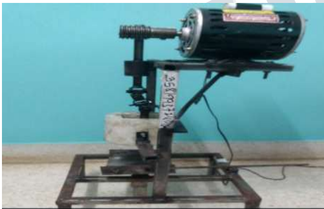
Fig 8: side view of precession Square hole drilling
