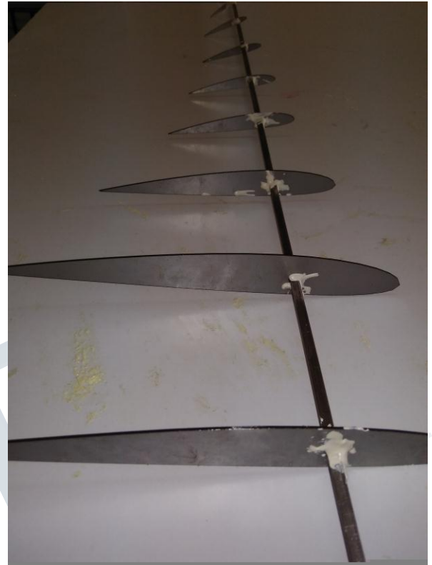
Fig 10: Skeleton structure of blade
