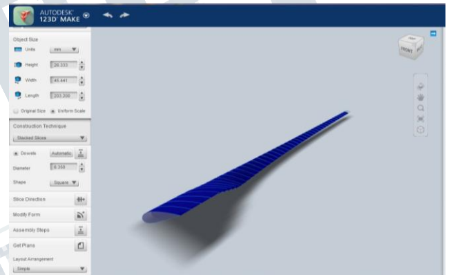
Fig 8: Blade sliced into 10 parts
