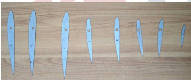
Fig 9: Blade profiles after laser cutting
