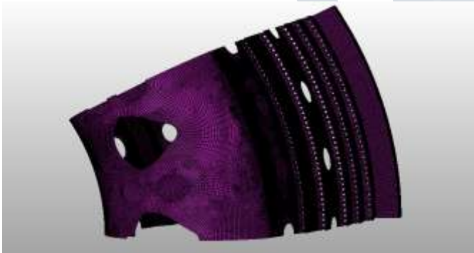
Figure 3: 3D FE Model of Combustor Chamber Liner
