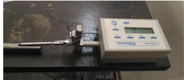
**Figure 7 Surface Roughness Tester**
