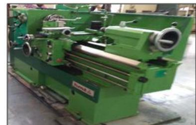
**Figure 1 HMT Lathe NH 22**
