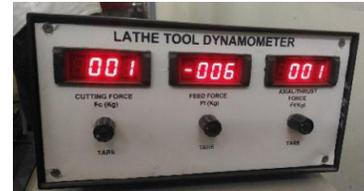
**Figure 4 Lathe Tool Dynamometer**
