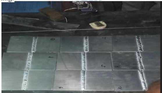
**Fig.4 Nine welded samples.**
