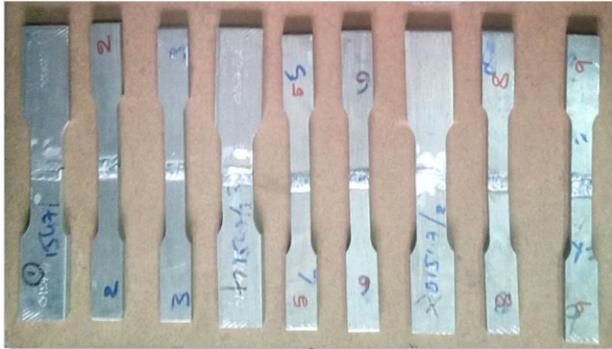
**Fig.7 samples prepared for tensile test.**
