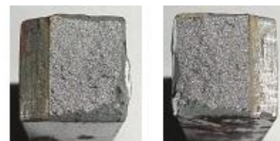
Fig. 3.4 Fractured surfaces of the impact specimen (Untreated)
