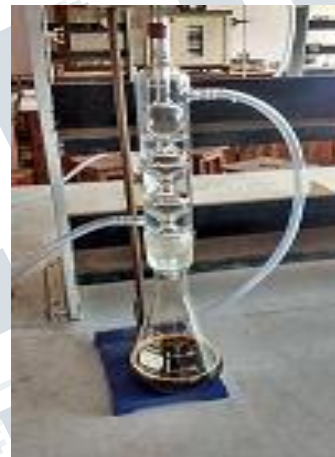
Fig 1. Typical experimental setup for corrosion rate measurement
