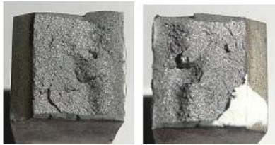
Fig.3.6 Fractured surfaces of impact specimen (NH 4 SCN treated)
