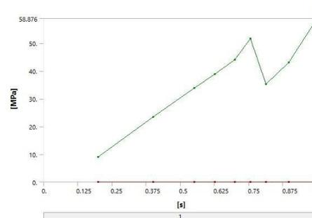
from the above results obtained it is observed that the minimum frictional stress at any instant of time is zero and the maximum frictional stress goes on increasing with in
