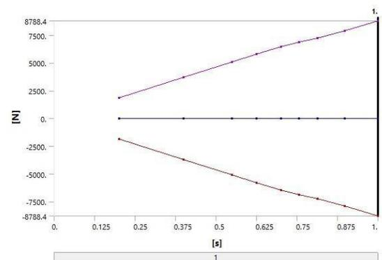
From the above results it is observed that the pressure increases as the delamination takes place and reaches the maximum value at the end of the contact region as it is clearly observed from the fig. 3.
