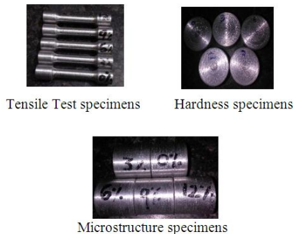
Fig. 3: Specimens prepared / machined for tensile test, hardness test and microstructure analysis
