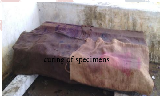
Curing Of Specimens
