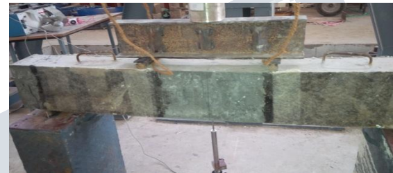
Ultimate failure of strengthened beam 1
