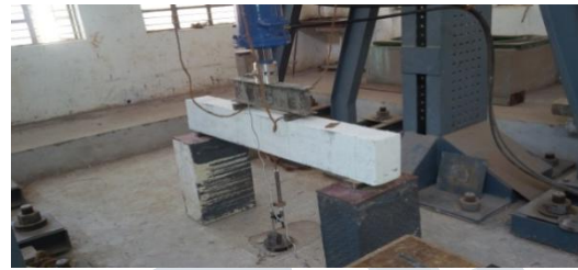
Experimental setup for testing of beams
