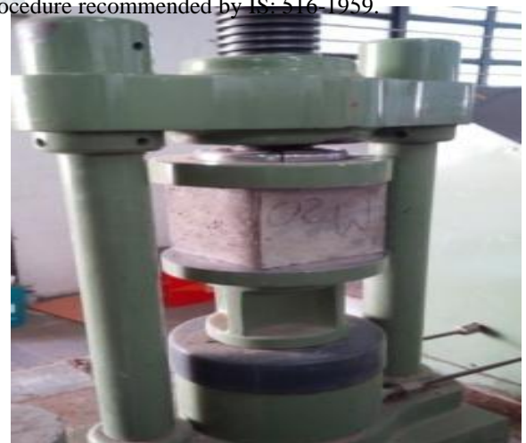
Testing setup of cube
