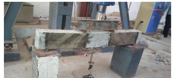
Test setup strengthened beam 2
