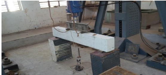
Test setup of control beam
