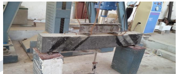
Test setup of strengthened beam 4
