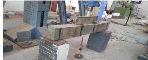
Test setup of strengthened beam 1
