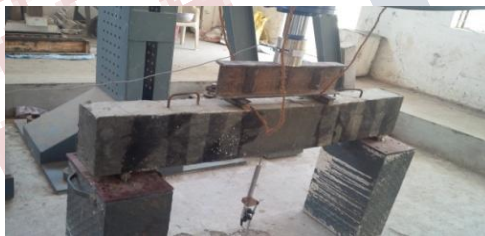
Test setup of strengthened beam 3
