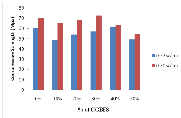
Figure 1. Optimum compressive strength at 0.32 and 0.30 w/cm ratio.
