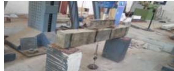
Test setup of strengthened beam 1
