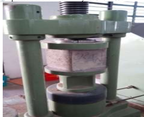
Testing setup of cube
