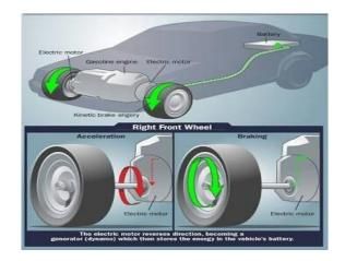
When the driver steps on the brake pedal of a vehicle, these types of brakes put the vehicle"s electric motor in reverse mode, causing it to run backwards, thus slowing the vehicle"s wheel. While running backwards, the motor acts as generator thus producing electricity. In this working model during braking the electric motor will be in contact with the drum, which in turn produces electricity. The produced power will be fed into batteries for later use or used immediately.
