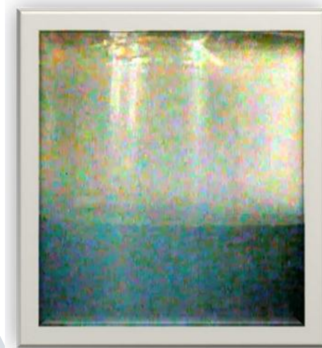
Figure3: Acrylic Container filled with glycerol and silicon carbide in the ratio 80:20 by volume fraction
