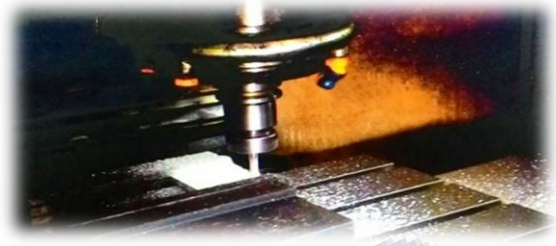
Fig.5. Setup while machining SMC
