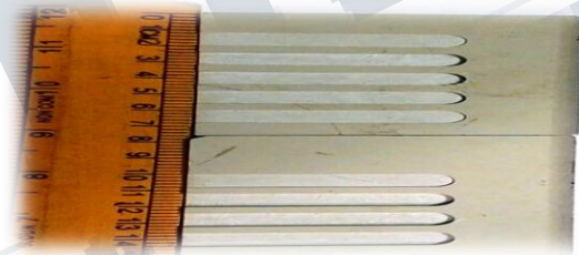
Fig.6. SMC material after End milling
