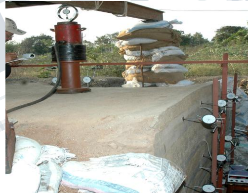
Plate 2. Observations during cyclic loading and built-in soil cement facing deformation of constructed model MSE wall.
