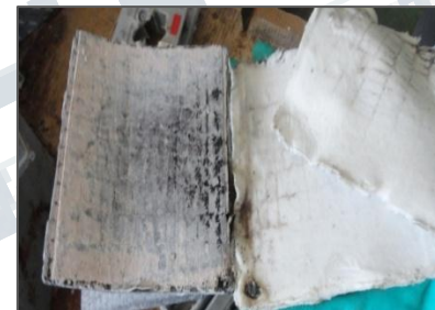
Improper conversion of plates due to Paste lump Photograph of defect part
