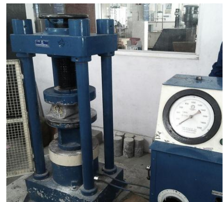
Fig 2.7: testing of cylinder for split tensile strength
