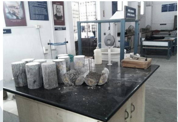
Fig 2.6: Cylindrical specimen after split tensile strength test.
