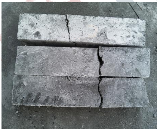
Fig 2.5: Concrete beam after testing in flexural testing machine
