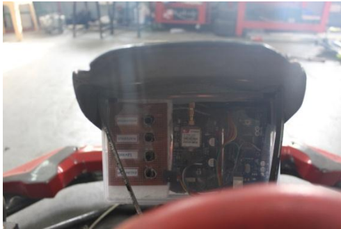
Fig 4.3 Transmitting system in go kart vehicle
