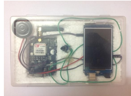
Fig 4.5 Receiving system for go kart vehicle
