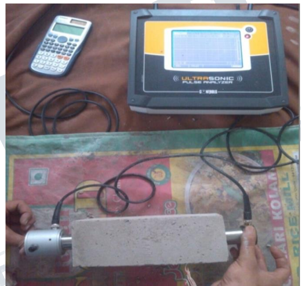
Fig. 4. Ultrasonic Pulse Velocity testing of adobe bricks
