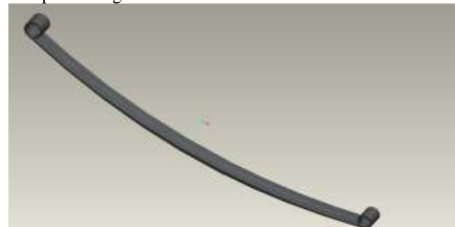
Fig. 4 Model of EN47 Leaf Spring in Pro-E 4.0
