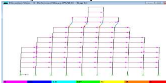
Fig 3.8: Deformed Shape and Hinge formation IRS-1
