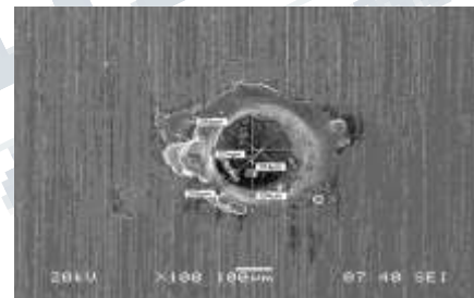
Fig. 3: SEM photograph at process parameters: P_w = 700 \mu\text{s} , P_f = 3 , P_{av} = 2 \text{ W} , air flow rate = 5 lit/min, time = 20 sec.
