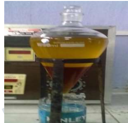
Fig. 3 Settling after base treatment
