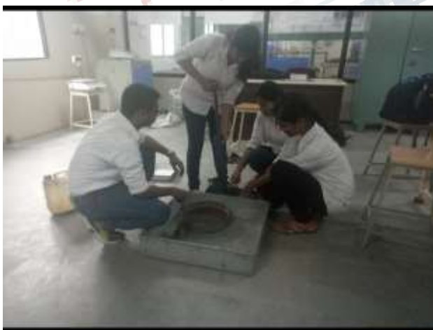
Fig. Performed Standard Proctor Test on BC Soil
