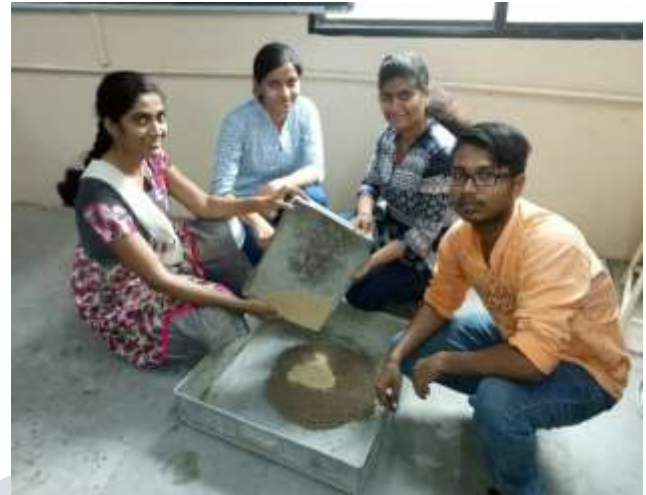
Fig. Mixing of Rice Husk Ash with Soil
