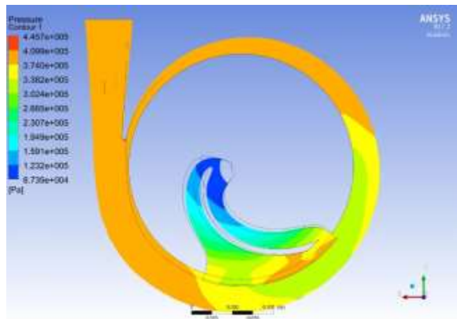
Fig. 10: 65% fly ash slurry 38 cubic meter per second
