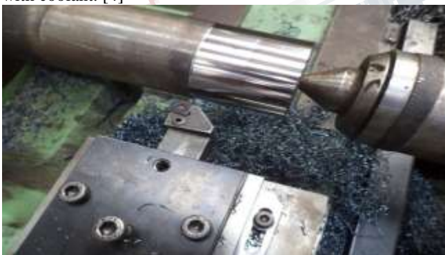
Figure No.2.1 Setup for Turning
