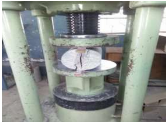
Figure 4: Setup in split tensile test
