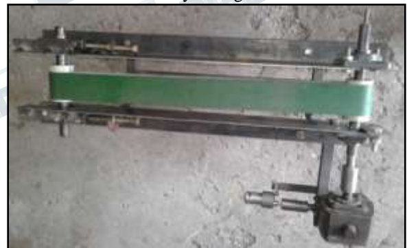
Fig: 4.1 Assembly of Belt Conveyor shaft
