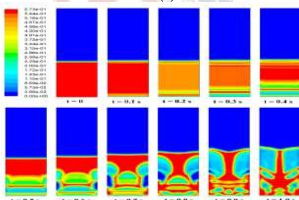
**Figure 4. Solid volume fraction contour from 0 to 1 s.**
