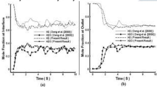
**Figure 3. Molar fraction in gas phase along the centerline of the reactor ( $x = 12.5$  cm) and (a) at height of 30 cm of inlet and at (b) outlet**
