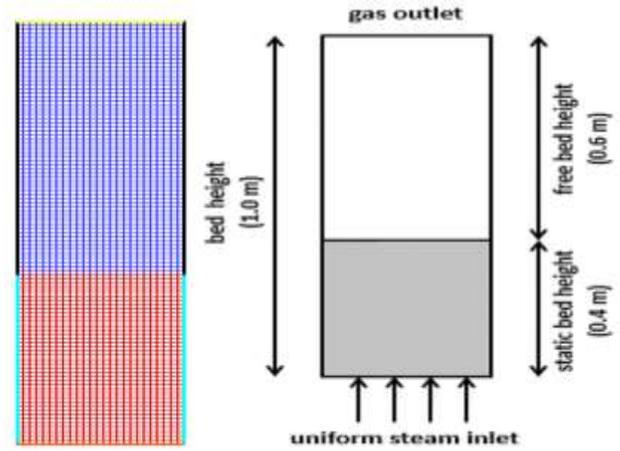
Figure. 2. Schematic and grid of the steam reactor.
