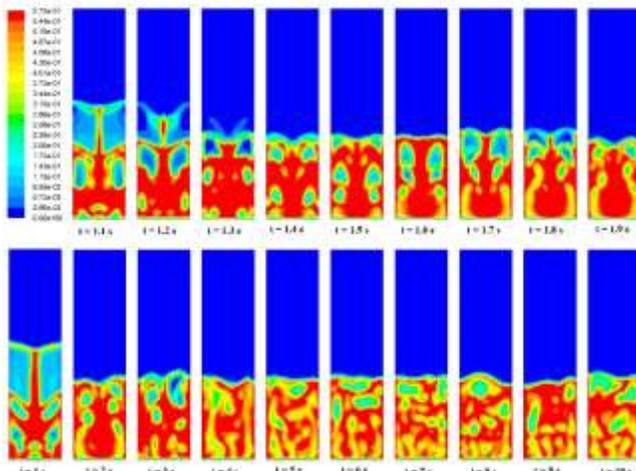
**Figure 5. Unsteady and quasi-steady development of solid volume fraction contour**
