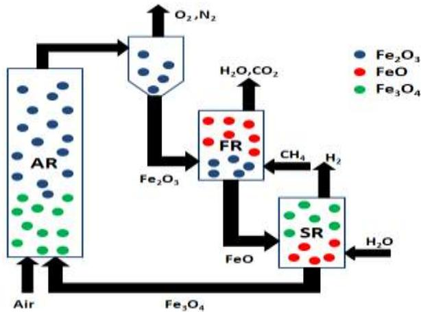
Figure.1. Schematic of three reactor chemical looping reforming process.
