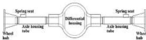
Fig.4 : Application of axle drive shaft (Ref.3)
